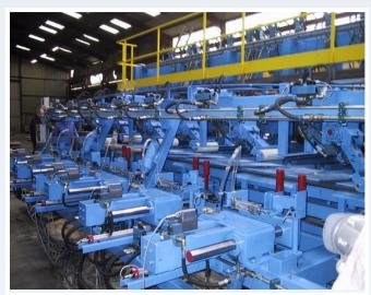
A 4 shifting saws edger can produce 3 different squared boards
