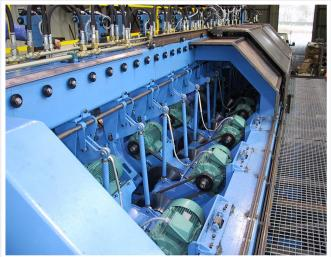
After trimming, 2 different wany boards can be loaded simultaneously onto the infeed table and independently optimized depending on the taper and the profile of each individual baord.
