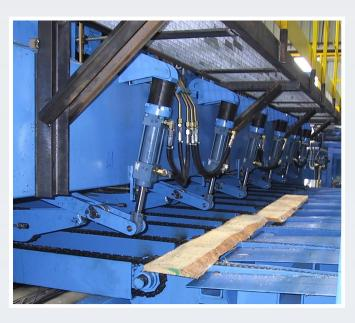
Thanks to the numerical multi-pinstops infeed table, 2 wany boards can be loaded together and tapered independently before edging one by one.
