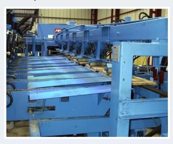
Vue inside a 4 shifting saws edger equiped with 1 fixe size extra saw on each side.
