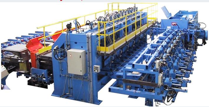
EGA Scanner: The full shape 3D scanner measures in real time the exact profile of each baord at a speed up to 40 bords per minute. Thanks to the knowlege of the board's and wane profile, the EGA optimizer calculates in one instant the best trimming (or length recutting) and boards edging taking into account the recothe \$ value of each finished products.
