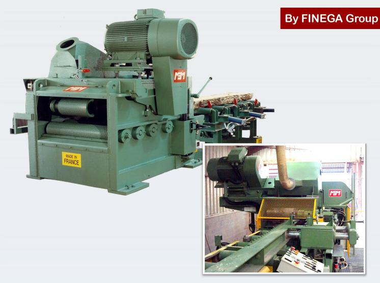
This multi-blades with circular saws is part of the COBRA range and uses the technology of sawing in the feed, with overhead saws. This machine is intented to cut 2,3 and 4 sided cants, of soft wood and hardwood .
