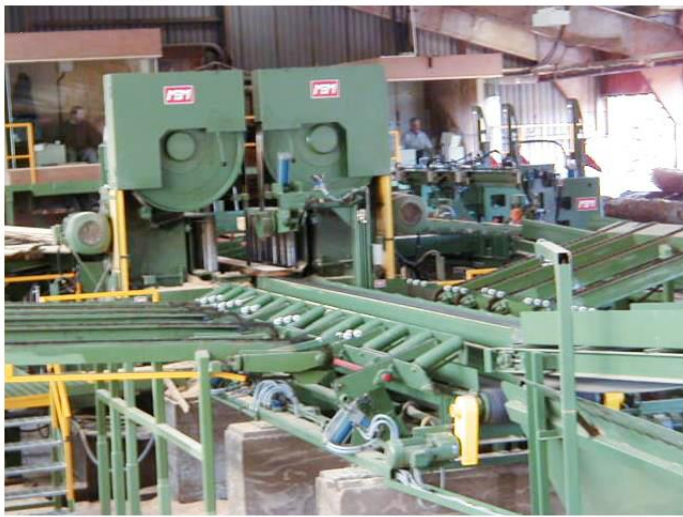
Outfeed, separating devices and waste collector designed to every customer needs
